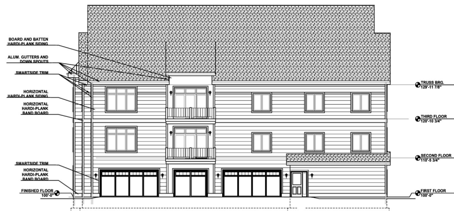
Building Elevation from Garage/Parking and Building Entry (Western Exterior Elevation)
